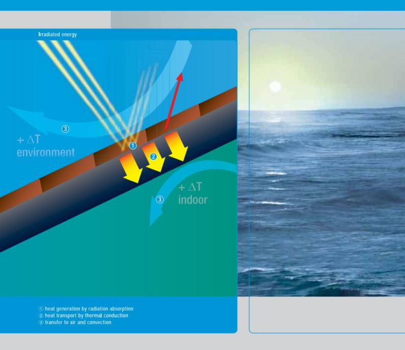
The energy radiated by the sun hits the colored surface. When the radiation is absorbed, this generates heat, which is transported by thermal conduction into the material and by convection into the surrounding air. Less absorption automatically means less heat build-up.
